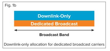
LTE-based 5G Terrestrial Broadcast could be deployed in any mobile downlink band including SDL (supplemental downlink) bands, for example the L-band (1452–1492 MHz).
