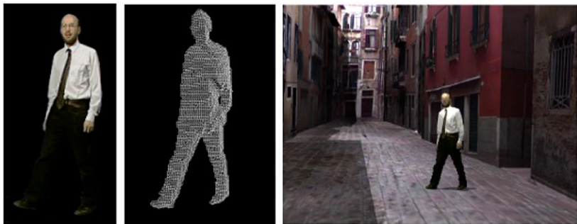
Figure 5. Example of 2.5D capture where an actor is recorded, segmented from the background (left), reconstructed in 2.5D (middle), and teleported into a 3D environment, including shadow casting and relighting (right).
